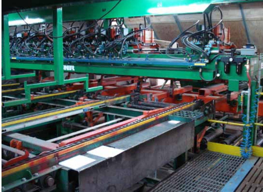
Above and left: What was originally a bellcrank-actuated sawmill stacker was modified to become a high speed, low profile dry mill stacker, equipped with a lineal cylinder-actuated fork system.
