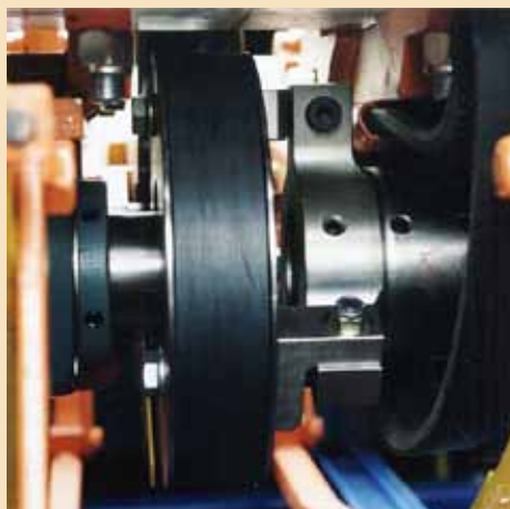
Below: The quick change coupling is standard on all new USNR trimmers, and can be retrofitted to existing lineshaft trimmers.
