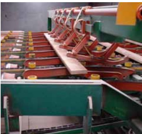
Below: Cut-n-two clamps lift boards into empty lug spaces at the outfeed of the trimmer.
