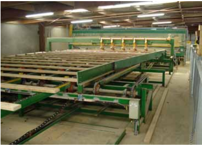
Above left and right: The trimmer line flows directly level into the redesigned sorter infeed.
