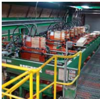
A new vacuum lath placer features 8 pairs of adjustable width magazines to accommodate varying package widths.
