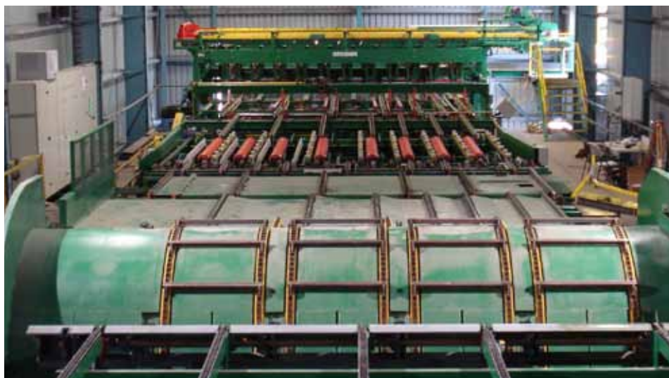
A new stacker with slant hopper stick placer accommodates the mill’s requirement for pre-course makeup, course gapping, and larger packs, all features that were not available with the used stacker.
