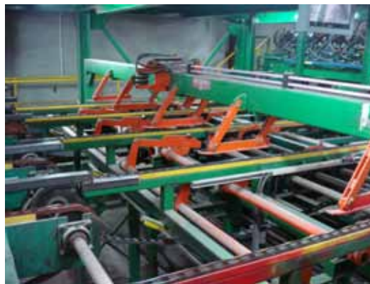
Above and left: What was originally a bellcrank-actuated sawmill stacker was modified to become a high speed, low profile dry mill stacker, equipped with a lineal cylinder-actuated fork system.
