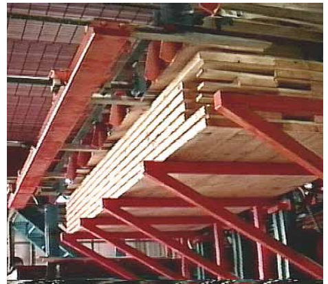
Above right: Tier skewing can increase package stability when making solid lumber stacks.
