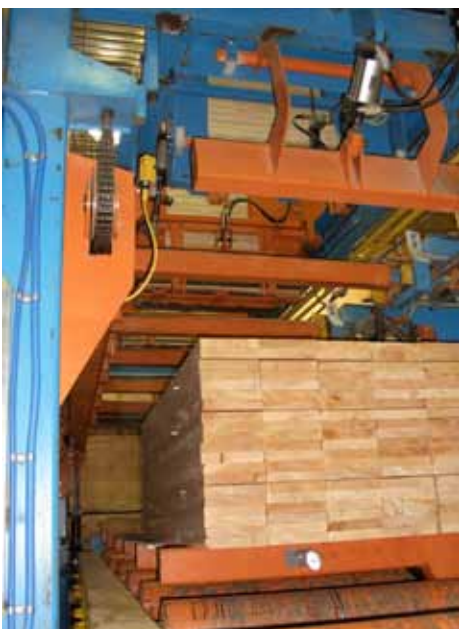
Above left: End tamping ensures lumberline end of package is square and even.
