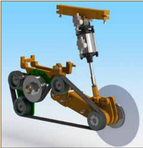
Above: The 'S' drive belt arrangement is a recent offering for new machines and a conversion for existing lineshaft trimmers.
