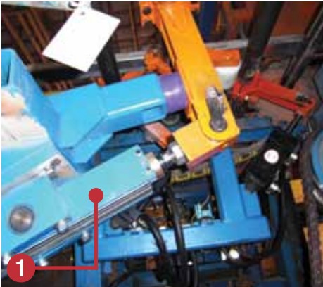
1. Exlar motion control cylinder actuates the forks' up and down movement.
