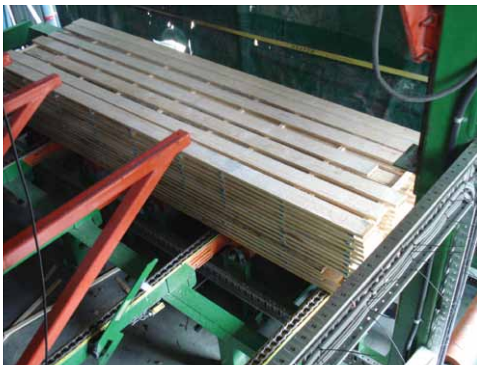
Course gapping is one of the features the mill incorporated into their new stacking system to facilitate drying thicker products.
